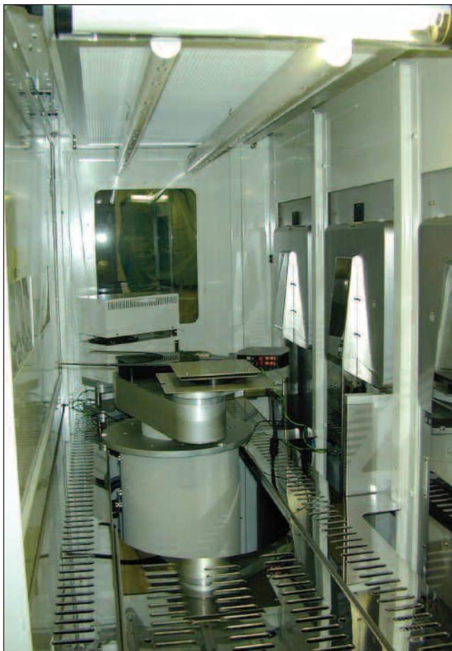
**Figure 3:** Ionization bars installed below the fan filter face of the ULPA filter in the equipment front-end module.
