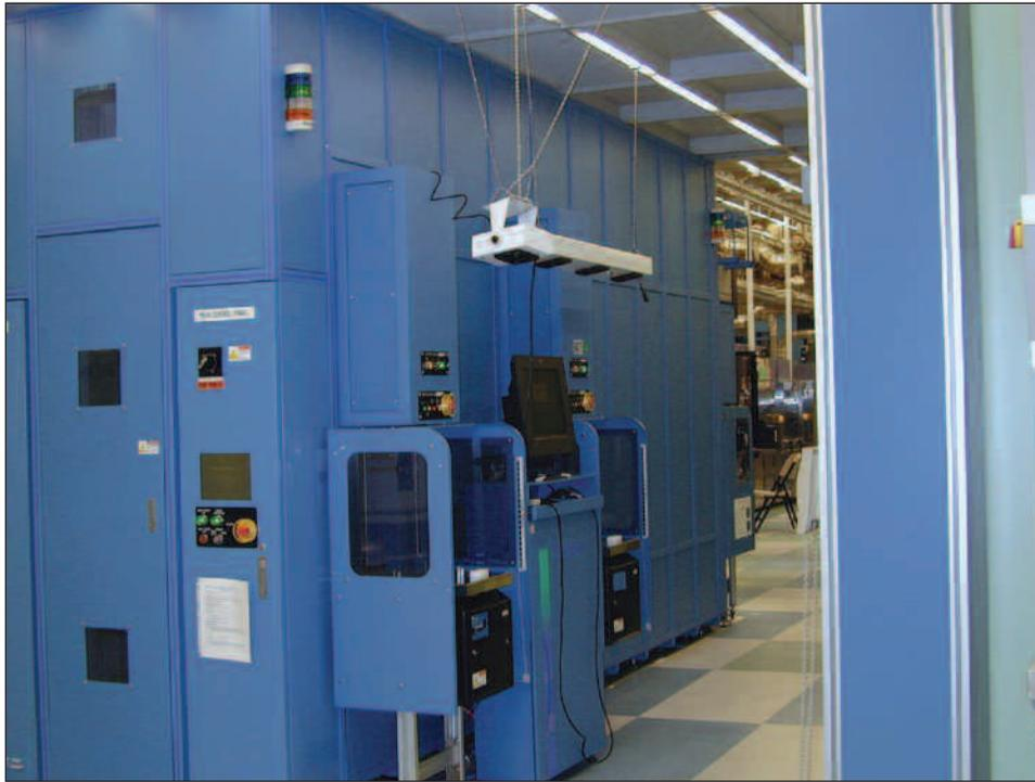
**Figure 2:** FOUP stocker with spot air ionization used for neutralizing the pod before uploading.
