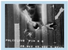
Figure 2. Typical damage to semiconductors (Above) and disk drive heads (Below).
